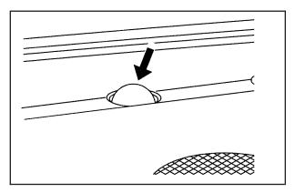
There is a solar sensor located on top of the instrument panel, near the windshield.
